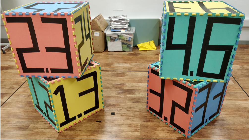
Figure 7.8: A photograph of the double towers scene. It contains two stacks of rotationally offset foam boxes separated by a distance of less than 1 m.
