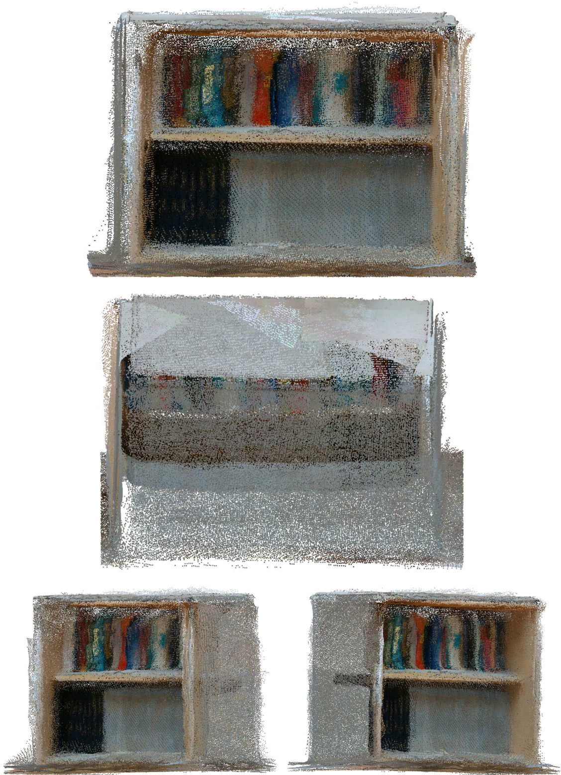
Figure A.18: The RGB coloured pointcloud result obtained from an observation of the small bookshelf scene using SEE++ with the Intel RealSense D435.
