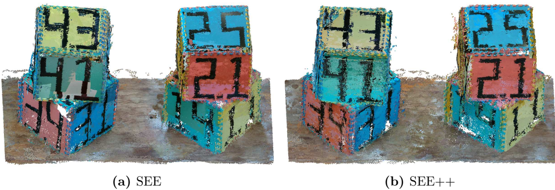
Figure 7.9: The RGB coloured pointcloud results obtained from observations of the double towers scene using the Intel RealSense D435 with SEE and SEE++.
