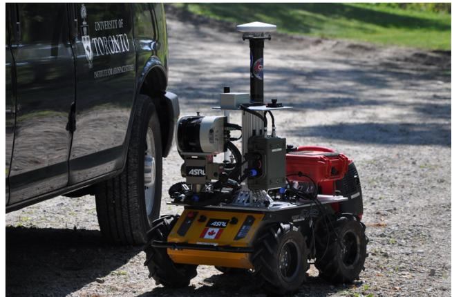
**Figure 1.** The ASRL Clearpath Husky A200 equipped with a laser rangefinder, star tracker, and inclinometer.
