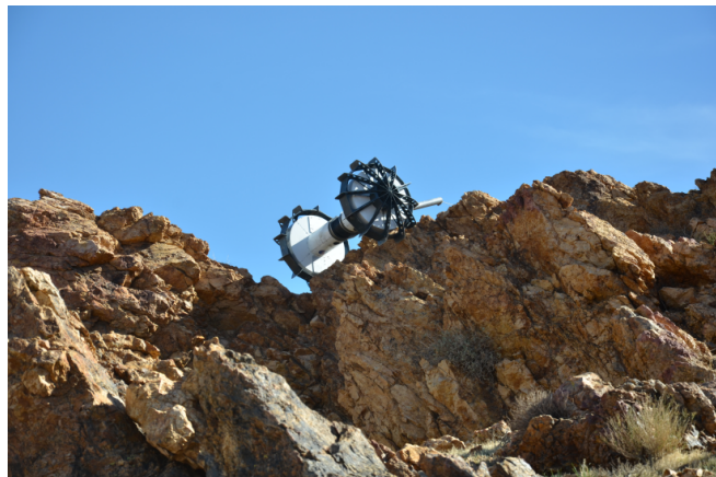
Fig. 1: The JPL Axel rappelling rover traversing rocky vertical wall in a Martian analogue site in Mojave, CA. Rappelling rovers are capable of delivering large payloads to steep surfaces.
