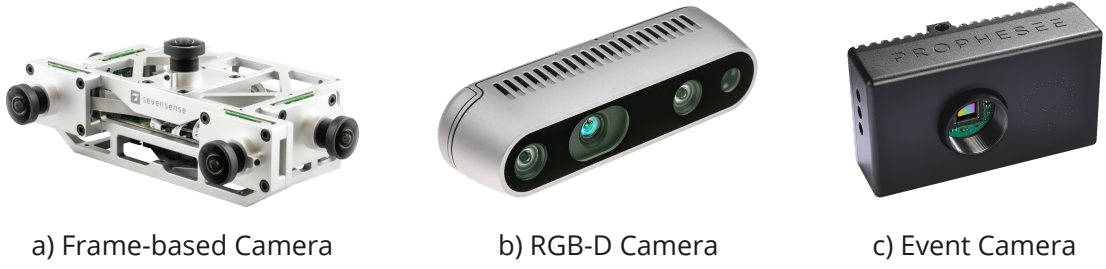
Figure 2.4: Vision sensors used in the works presented in this thesis. a) shows an example of frame-based camera—Sevensense Core Research multi-camera visual-inertial sensor (Source: Sevensense [224]). b) is a Realsense D435i RGB-D camera (Source: Realsense [107]). c) is a Prophesee event camera without a lens attached (Source: Prophesee [196]).
