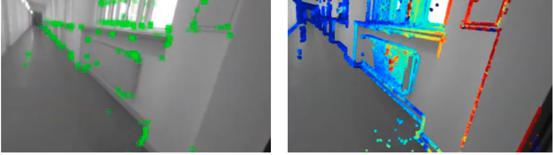
Figure 3.1: Comparison between feature-based and direct frontend. Left: Sparse corner features are extracted and tracked between images, and the pose can be estimated by minimizing the reprojection error using the feature tracklets. Right: Direct method computes the photometric error of the image intensities between frame for pose estimation.
