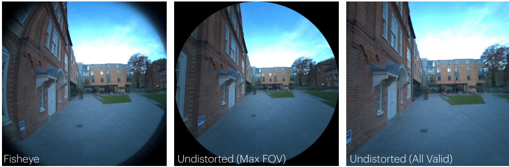
Figure 8: We provide three image types: the original fisheye, a Max FOV undistorted version with wider coverage and black borders (with a valid pixel mask provided), and an All Valid version with no black borders but a smaller field of view for easier use.
